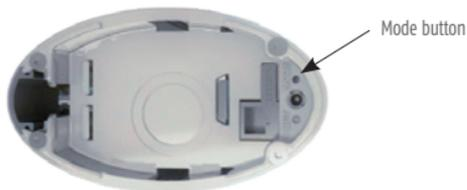
Press and hold the Mode button until the Yellow LED turns off.
