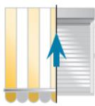
Briefly press the **my** and Up buttons simultaneously. The product will begin to move up and tension against automatic lock.
