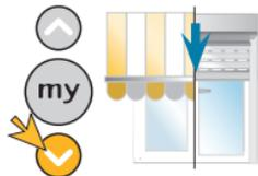
Press the down button continuously until the lower limit is reached. The motor will continue to travel down if held for more than 2 seconds.
