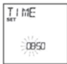
TIME and SET will appear on the display. Use the navigation button to set the current hour time (24 hour clock).
