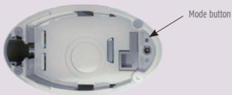
Press and hold the Mode button until the Green LED turns off.
