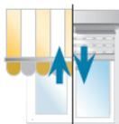
Press and hold the Up and Down buttons for 7 seconds. The motor performs a jiggle and then a second slower jiggle.
