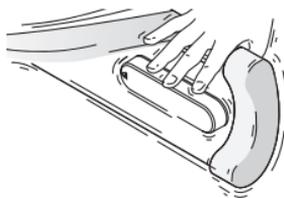
Test the sensor functionality by shaking the awning.
