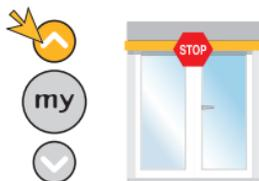
Press up and stop the product at the Up limit position. Press the corresponding limit button on the motor until the button springs up.
