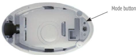
Press and hold the mode button until the Green LED turns off. The motor direction has been changed.
