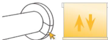
Press the program button on the motor until it jiggles.
