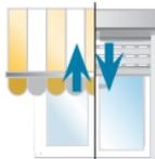
Press and hold the Up & Down buttons for 7 seconds. The motor performs a joggle and then a second slower joggle.
