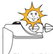
Trigger the light threshold by shining a torch on the sensor lens – the product will extend after approximately 10 seconds
