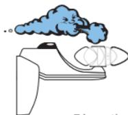
Trigger the wind threshold by blowing hard on the sensor wind cups – the product will retract almost immediately
