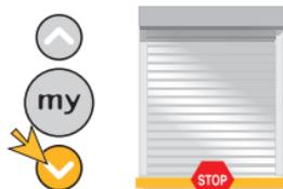
Press down and stop the product at the Down limit position. Press the corresponding limit button on the motor until the button springs up.
