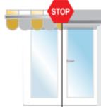
Press the Up button continuously until the upper limit is reached. The motor will continue to travel if held for more than 2 seconds.
