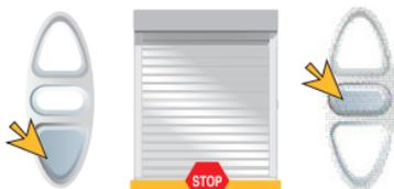
Power the motor down and stop the product at the Down limit position. Press the corresponding limit button on the HiPro motor until the button springs up.
