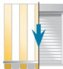
Press and hold the **my** and Down buttons on the transmitter. The motor will start to move down. Release the **my** and Down buttons to stop the motor below the locking mechanism. Click or lock the bottom bar in place.
