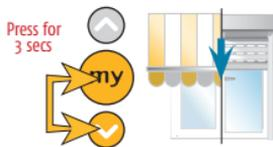
Move the motor to the desired position using the Up or Down buttons.
