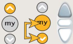
Control button operation - The yellow or grey button images along with the yellow pointing arrow require the installer to push the corresponding buttons as illustrated in the guide. Where highlighted, there may also be a requirement to hold the buttons for a set time period e.g. - **Press for 3 secs** - This would require the installer to press and hold the relevant button(s) for up to 3 seconds.
