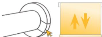
Hold the program button on the motor until the motor jiggles.
