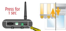
Press program button on the RS485 Transmitter for 1 second.
