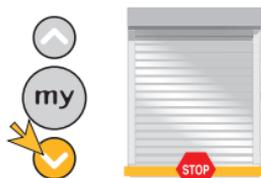
Press Down and then stop the product at the Down limit position. Press the corresponding limit button on the motor until the button springs up.
