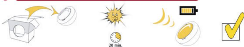
Before programming the sensor, remove it from the packaging and place it in direct sunlight with the solar panel up for a minimum of 20 minutes.
