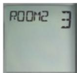
*Manual mode: Channel 3 is programmed to a motor/group of motors named "Room 2"*
