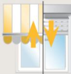
JIGGLE - The term 'jiggle' is used to describe a quick double movement from a Somfy RTS motor when it recognises a radio command and signals its response to the installer. In other words, you may signal a command to a RTS motor from a RTS controller and the end product (awning, roller shutter, blind etc.) will move briefly back & forth or up & down to confirm the command.
