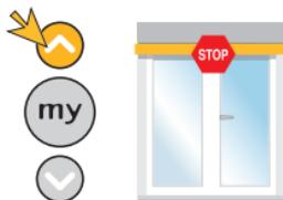
Press Up and then stop the product at the Up limit position. Press the corresponding limit button on the motor until the button springs up.
