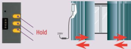
Press and hold the Open (up), Stop and Close (down) buttons simultaneously on the DCT setting tool or a dry contact switch until the motor jiggles once.
