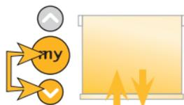
Hold the **my** and Down buttons until the motor jiggles.
