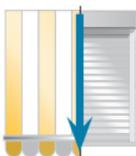
Position the screen at the desired lower limit, just below the manual lock.
