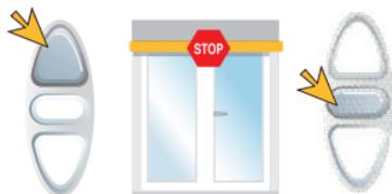
Power the motor up and stop the product at the Up limit position. Press the corresponding limit button on the HiPro motor until the button springs up.
