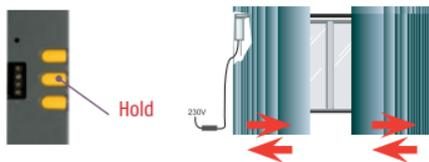
Press and hold the Stop button until the motor jiggles once. The motor direction has been changed.
