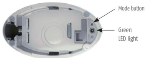
Maintain power on the motor in either direction and wait until the curtain stops. Press and hold the Mode button until a Green LED appears.
