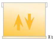
Hold the program button on the motor head until the motor jiggles 3 times.
